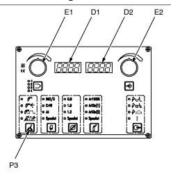
Set Manual MIG welding process using P3 push button.
